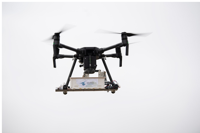
Image 2: AUSEA gas analyser mounted on a drone, developed by TotalEnergies and its R&D partners
